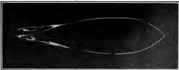
FIG. 18. FLOW FOR FINE STRUT.
